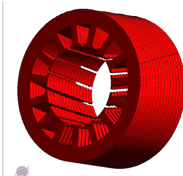
Figure 9: Approximation of skewed motor by piecewise-skewed stator.
