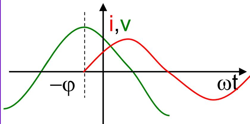
$$v(t) = L \frac{d}{dt} i(t) = L\omega\sqrt{2}I \cos(\omega t + \varphi + \frac{\pi}{2})$$
