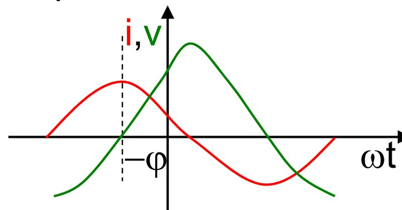
$$v(t) = \frac{1}{C} \int_0^t i(t') dt' = \frac{1}{\omega C} \sqrt{2} I \cos\left(\omega t + \varphi - \frac{\pi}{2}\right)$$
