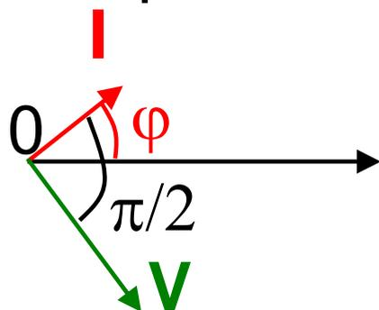
$$\begin{aligned} \mathbf{V} &= -\frac{j}{\omega C} \mathbf{I} \\ &= \frac{I}{\omega C} \angle \varphi - \frac{\pi}{2} \end{aligned}$$
