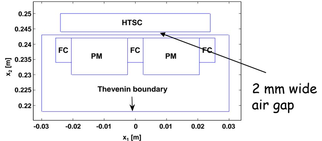
The HTS sample (48 mm times 6 mm) is supposed to be in the **zero-field state**; accordingly, it is modelled as a **perfectly diamagnetic** material.
