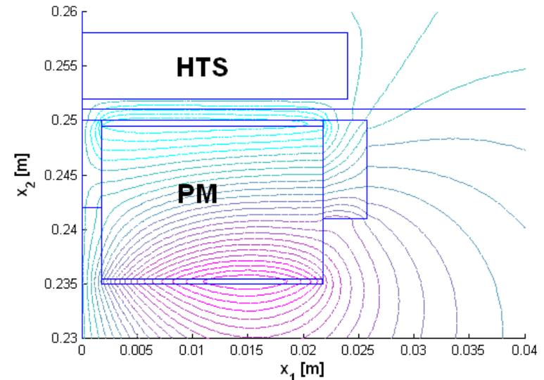
Final geometry with flux lines
