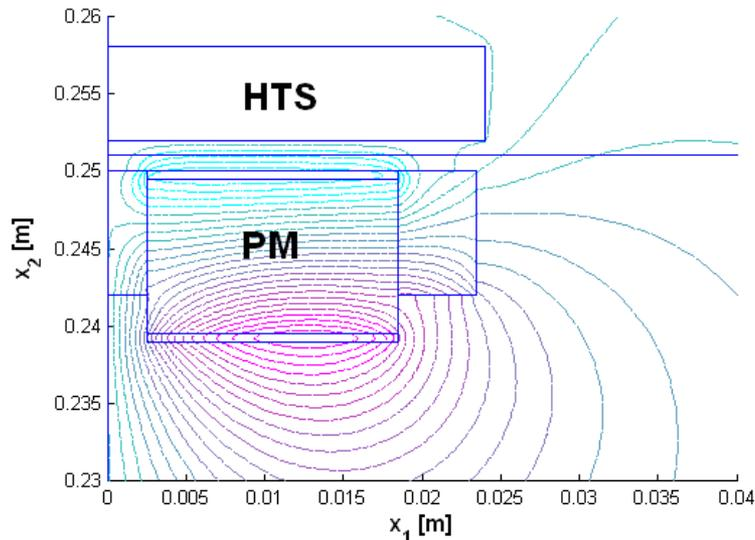
Initial geometry with flux lines
