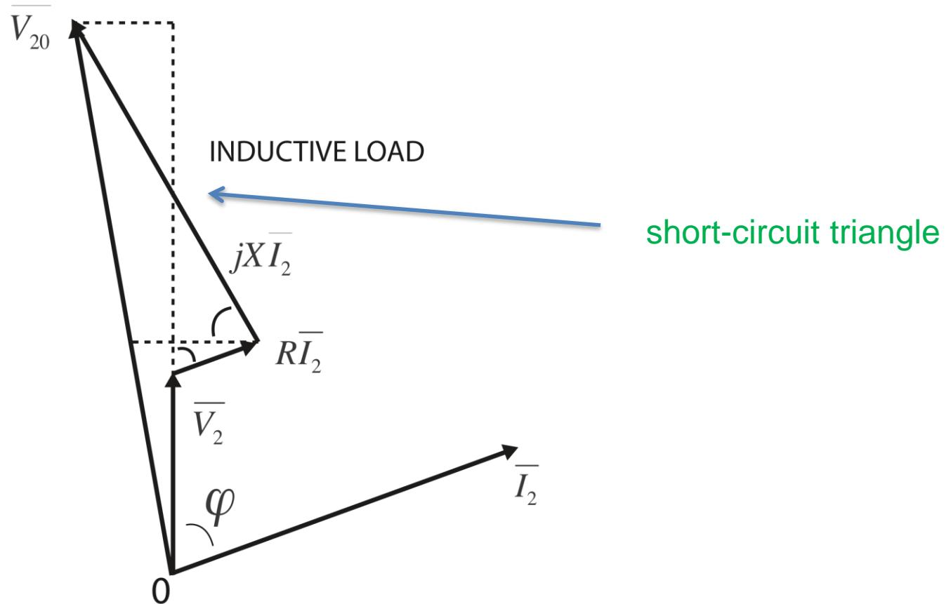
$$\Delta V \equiv V_{20} - V_2 \simeq RI_2 \cos \varphi + XI_2 \sin \varphi$$
