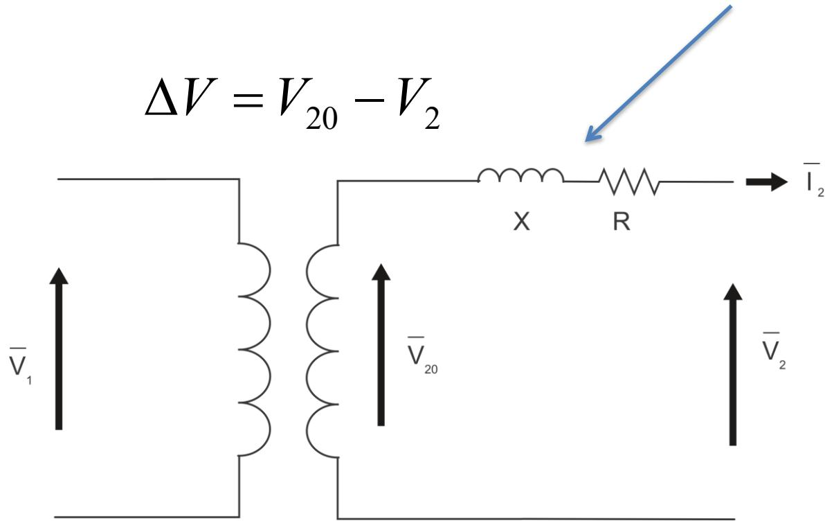
$$\frac{1}{k} \bar{V}_1 = \bar{V}_{20} = \bar{V}_2 + (R + jX) \bar{I}_2 = V_2 + (R + jX)(I_2 \cos \varphi + jI_2 \sin \varphi)$$
