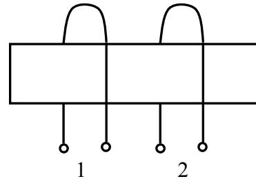
open magnetic circuit ( $f > 20 \text{ kHz}$ , core made of  $\text{Fe}_2\text{O}_3$ )
