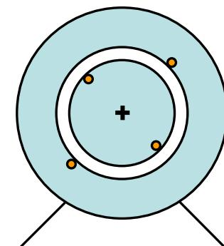
The rotor experiences a torque  $C=2RF_t$ : if unconstrained, it rotates.
