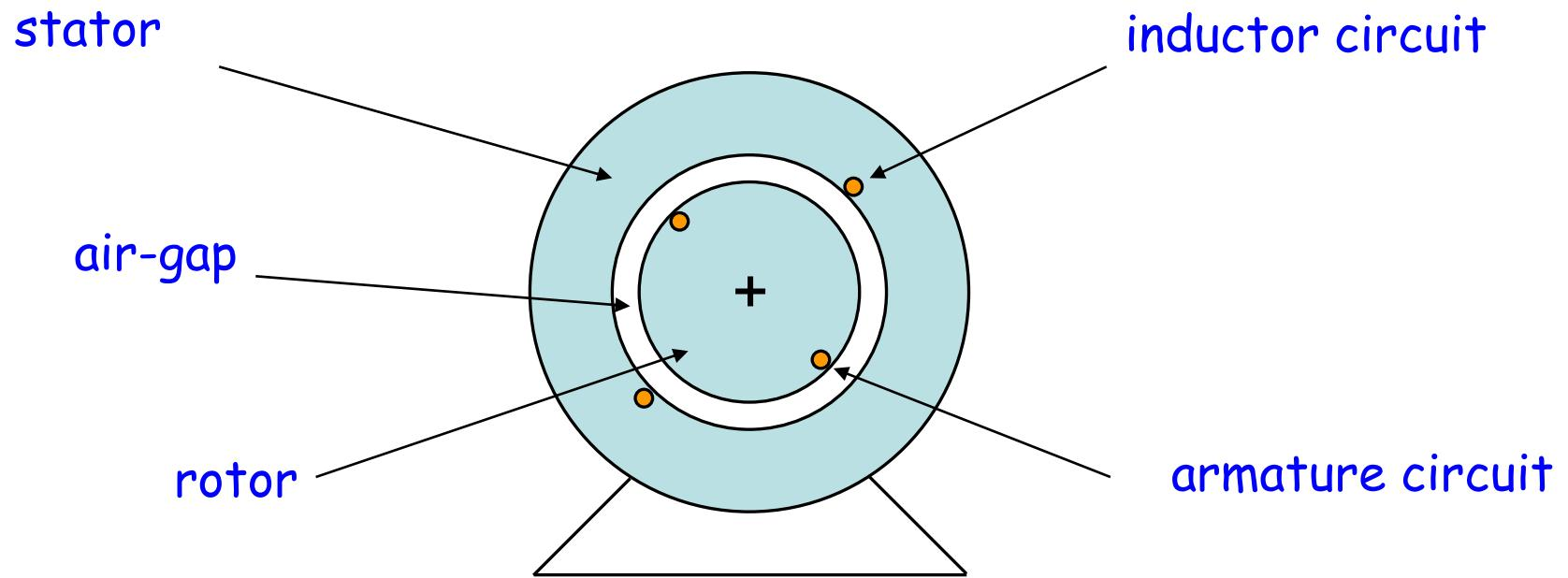
stator + air-gap + rotor = magnetic circuit
