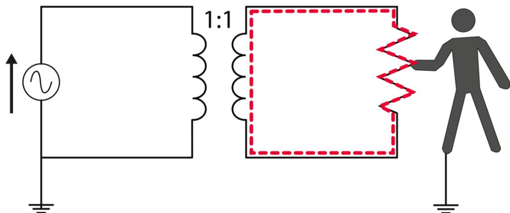
In this case the human body is safe: in fact, it does not close any circuit and, therefore, no current can pass through it.
