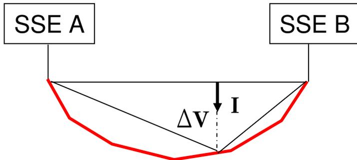
$$\Delta V = r x I_A = r I (x - x^2/L) \quad \text{andamento parabolico}$$
