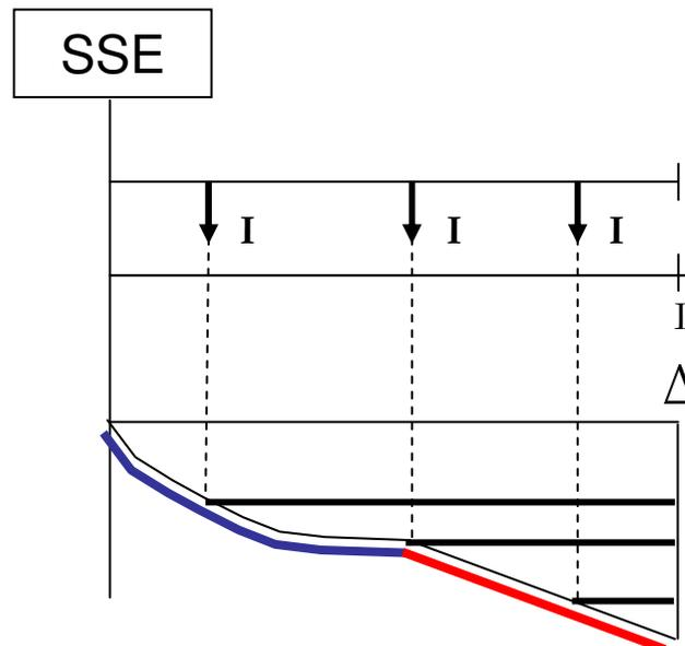
$$\Delta V_m = \frac{rI}{L} \left[ \int_0^{L/2} x dx - \frac{1}{L} \int_0^{L/2} x^2 dx + \int_{L/2}^L x dx - \frac{L}{4} \int_{L/2}^L dx \right] =$$
