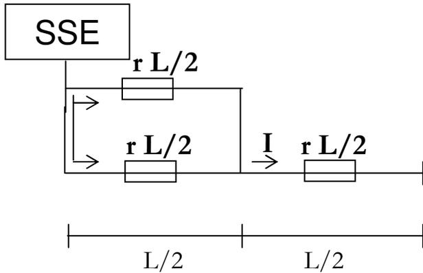
$$\Delta V = r I_1 x = r I (x - x^2/L) \quad \text{andamento parabolico}$$
