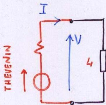
$$E_{TH} = E \frac{R_3}{R_1 + R_2 + R_3}$$
