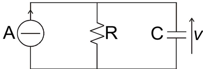
$$\begin{aligned} v_{x=0} &= \int_0^t e^{-\frac{1}{RC}(t-t')} \frac{A}{C} dt' = e^{-\frac{t}{RC}} \frac{A}{C} \left[ RCe^{+t'/RC} \right]_0^t \\ &= e^{-t/RC} \frac{A}{C} (RCe^{+t/RC} - RC) = RA(1 - e^{-t/RC}) \end{aligned}$$
