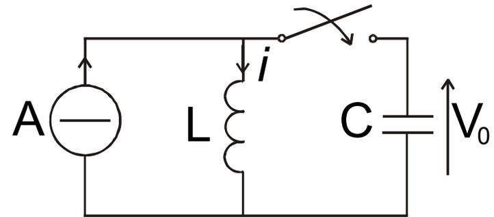
$$\left\{ \begin{array}{l} v(0^+) = V_0 = K \cos \vartheta \\ Dv(0^+) = -\frac{GV_0}{C} = -K\omega_0 \sin \vartheta = 0 \end{array} \right. \longrightarrow \left\{ \begin{array}{l} K = V_0 \\ \vartheta = 0 \end{array} \right.$$
