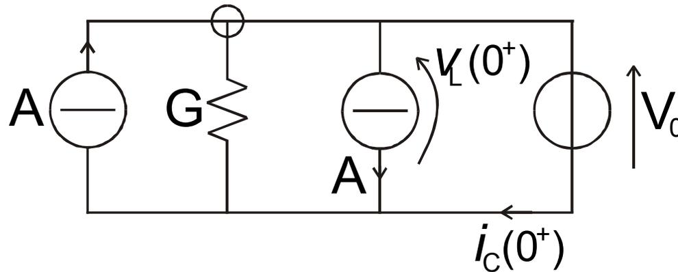
$$v_L(0^+) = V_0 \quad \longrightarrow \quad D i_L(0^+) = \frac{V_0}{L}$$
