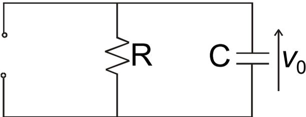
$$v_{u=0} = v(0)e^{tA} = V_0 e^{-t/RC}$$
