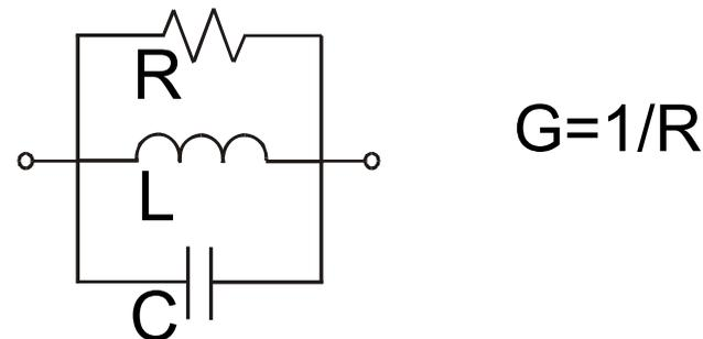
$$\mathbf{Y} = G + j\left(\omega C - \frac{1}{\omega L}\right) = \sqrt{G^2 + \left(\omega C - \frac{1}{\omega L}\right)^2} \angle \tan^{-1} \frac{\omega C - \frac{1}{\omega L}}{G}$$
