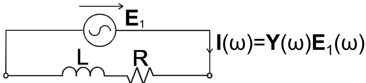
$$\mathbf{Z} = R + j\omega L = \sqrt{R^2 + \omega^2 L^2} \angle \tan^{-1}(\omega L/R) = Z \angle \varphi$$
