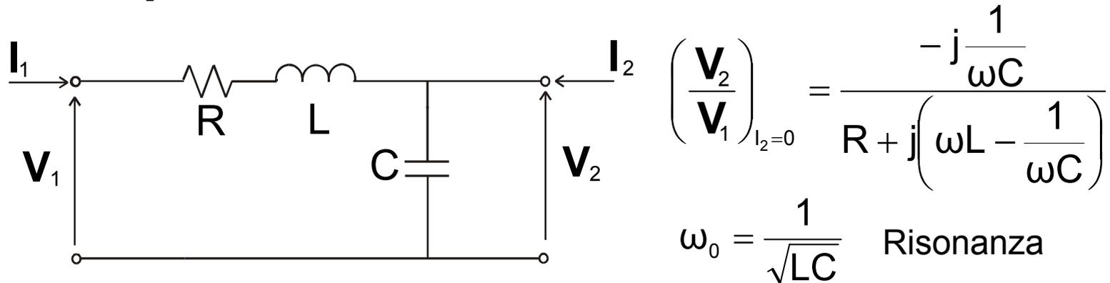
$$\omega \ll \omega_0 \quad \frac{1}{\omega C} \gg \omega L \quad \frac{1}{\omega C} \gg R \quad \left| \frac{\mathbf{V}_2}{\mathbf{V}_1} \right| \rightarrow 1$$
